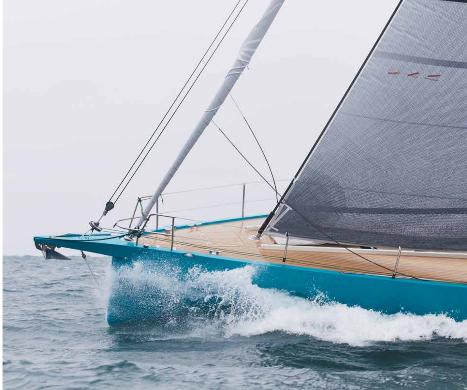
An epoxy glass-infused cockpit and deck keep Basyc lighter than an all-aluminium yacht
