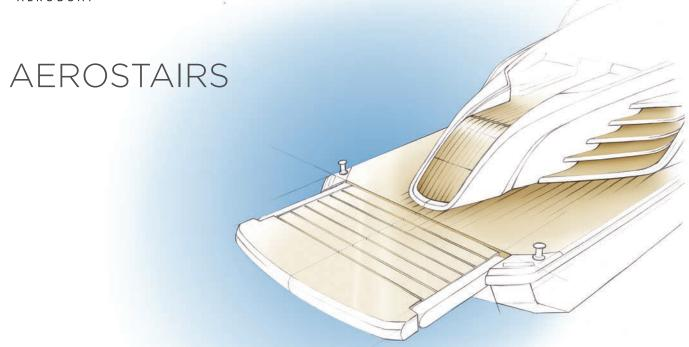
The Aerostairs is an extendable swim platform that can be raised for boarding and lowered to act as a beach club ladder. When combined with a wider than usual height adjustable passerelle stowed within the Superstructure Tail (and deployed automatically), the Aerostairs Platform becomes a one-of-a-kind boarding and disembarking system.
