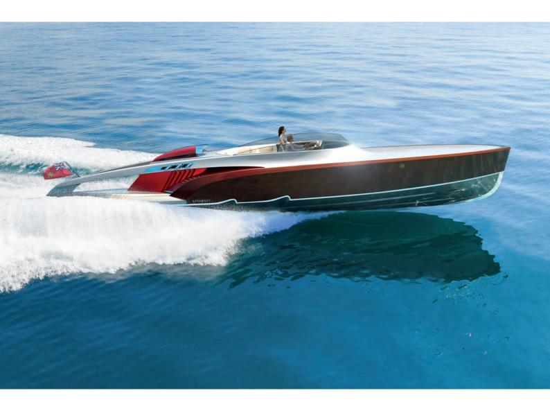
The first in the Aeroboat line is the 55ft SV12, powered by a reconditioned and fuel-injected Rolls-Royce Merlin V12 engine from a World War II Spitfire. While its Teardrop Cockpit features beautiful custom dials and landing-gear -inspired shock absorbing seats.
